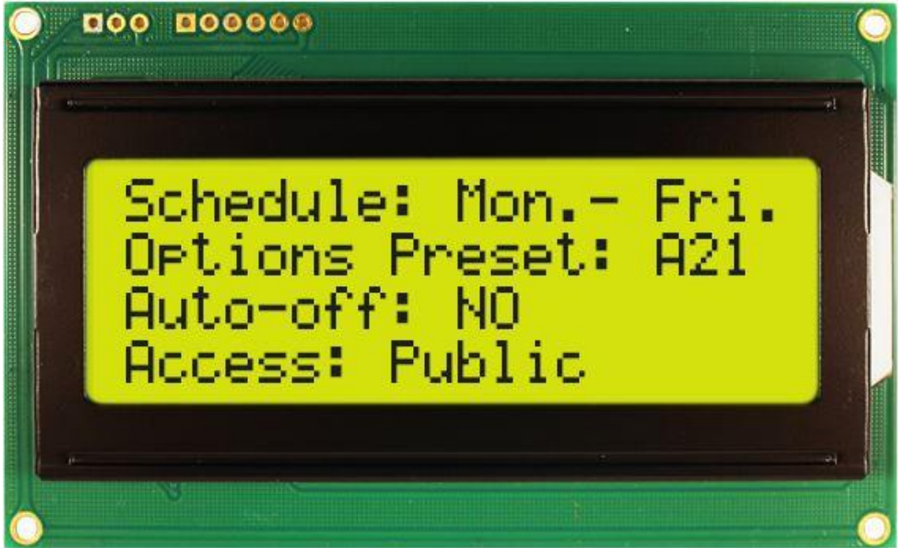
Figure 1: New heaven display NHD-0420D3Z-FL-GBW-V3
