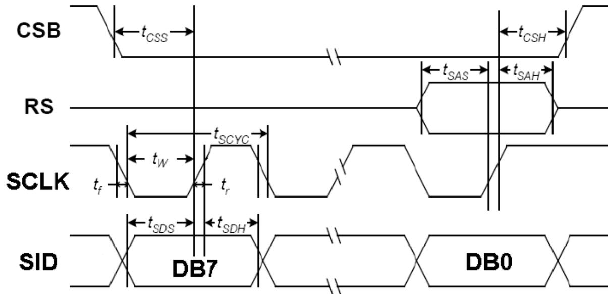
In 4-SPI Serial Interface (TA = 25°C, VCC = 2.7V )
