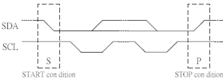
Fig .9.2 Definition of START and STOP conditions
