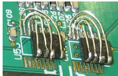
Figure 44: Patchwork of both SN75hvd12 level changers
